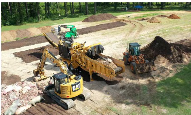
Simultaneous grinding of pig carcasses and co-compost material (Flory, 2022)
